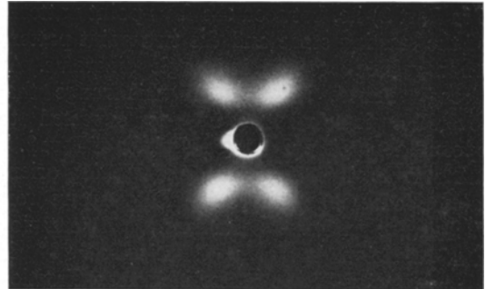
Figure 1d After extending A2 in the y direction at 98^\circ\text{C} . Extension ratio y/y_0 = 1.46 .
